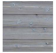
JAS "Small Knot" grade allows for up to 20 tight or 10 dead knots per 79" (2m) board length. Unlimited combination of heartwood and sapwood, pith allowed. Checks allowed to 1/16" as long as plank stability, weather-resistance, and cosmetics are not adversely affected.
