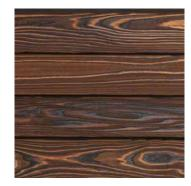
Premium Clear grade allows for up to 4 tight or 3 dead pinhole knots per 79" (2m) board length. Unlimited combination of heartwood and sapwood, no face pith allowed.
