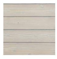
JAS "Small Knot" grade allows for up to 20 tight or 10 dead knots per 79" (2m) board length. Unlimited combination of heartwood and sapwood, pith allowed. Checks allowed to 1/16" as long as plank stability, weather-resistance, and cosmetics are not adversely affected.
