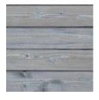
JAS "Small Knot" grade allows for up to 20 tight or 10 dead knots per 79" (2m) board length. Unlimited combination of heartwood and sapwood, pith allowed. Checks allowed to 1/16" as long as plank stability, weather-resistance, and cosmetics are not adversely affected.
