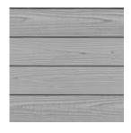
Premium Clear grade allows for up to 4 tight or 3 dead pinhole knots per 79" (2m) board length. Unlimited combination of heartwood and sapwood, no face pith allowed. Checks allowed to 1/16" as long as plank stability, weather-resistance, and cosmetics are not adversely affected.
