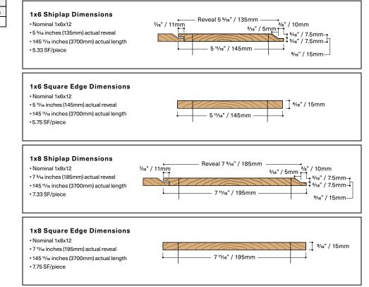
\*Dimensional shrinkage after manufacture is possible due to being a solid-sawn wood product.
