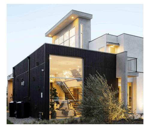
Yakisugi "shou sugi ban" siding and paneling. Original unbrushed charred surface, suitable for exterior and interior use. Exterior grade finish is not suitable for high-traffic applications. Interior grade finish is suitable for high-traffic applications. Delivered ready to install.
